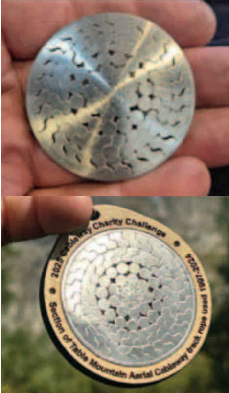
Successfully cutting the track rope into 3mm thick disks
